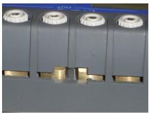
Connect your probes by simply pushing on the terminal top and insert wires of up to 3 mm or 10 AWG diameter and compensated thermocouple connectors. Wires are held tight between two brass plates ensuring thermal stability and a very good cold junction compensation for thermocouples.
